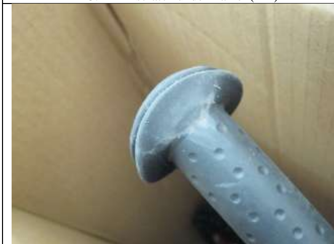
5. Right side handle rubber grip was unshaped
